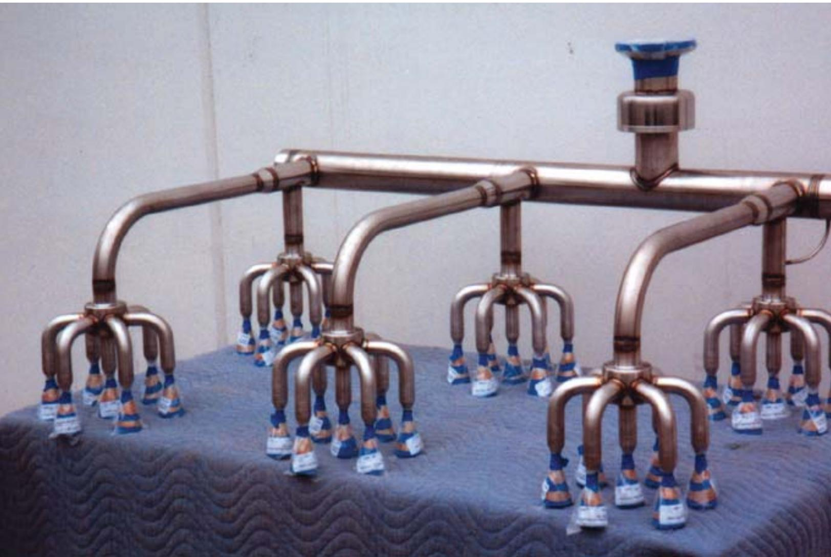
Dynamic Fabrication workers use an assortment of tools to create this Inconel manifold for the F-35's airborne laser program.
